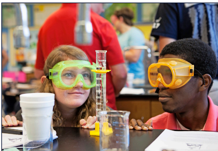
To determine the best substance to use in a handwarmer, Lauren Pearson and Vince Wynn are measuring a volume of water to find out the enthalpy change when lithium chloride and other substances dissolve in water.
